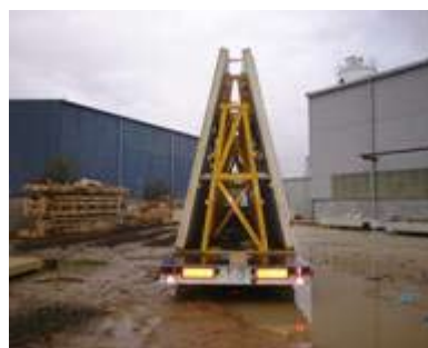
Panels on an A frame
